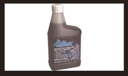
Kilfrost is a unique pneumatic anti-freeze and lubricant designed to provide meet the requirements of air powered tools. It provides lubrication to the moving parts, offers corrosion protection and prevents freezing of the condensation in the air lines. Kilfrost must be introduced into the air stream by an air line lubricator which will atomize the liquid and meter the flow.
